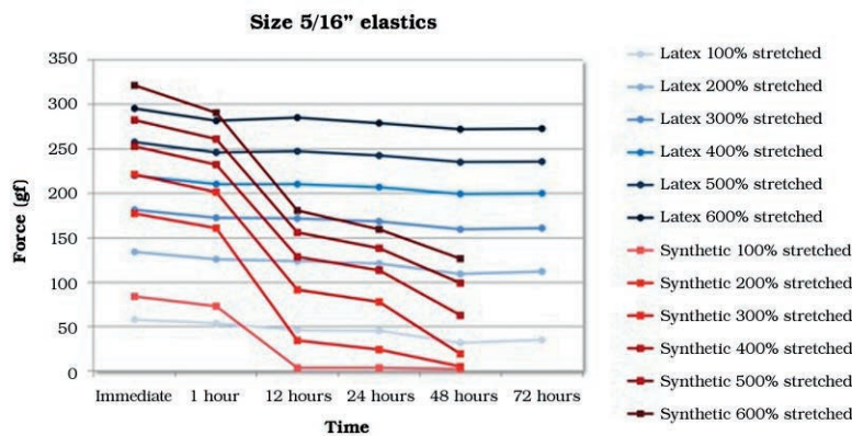
Figure 4 – Biomechanical dynamic behavior of the latex and synthetic size 5/16'' elastic over time, through the variation of the immediate mensuration up to 72 hour
