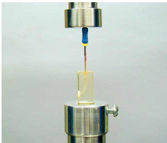
**Figure 2** - Set composed by resin block, gutta-percha point, and spreader positioned on the universal testing machine
