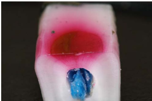
Figure 4 - Sectioned specimen aspect in order to make the dye infiltration analysis (left side control and right side test)
