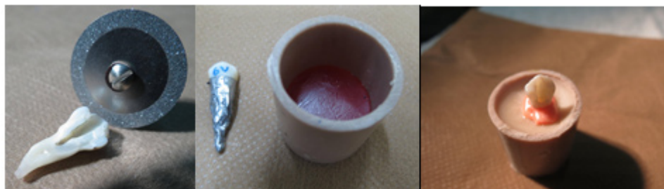
Figure 1 - Cutting of the roots and mounting in PVC rings
