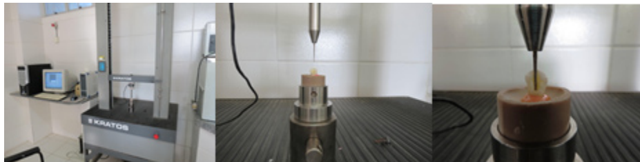
Figure 2 - Tooth inserted into the universal testing machine
