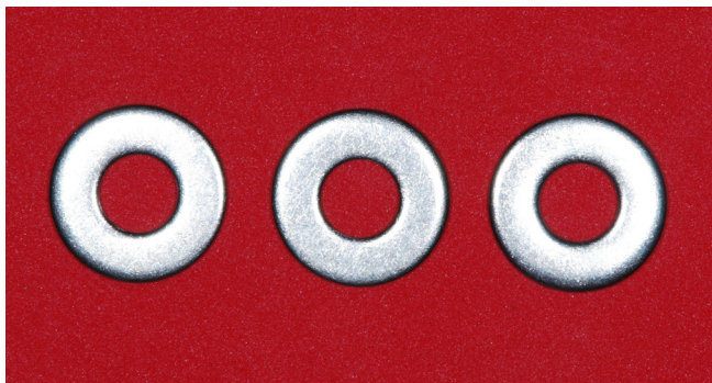
Figure 1 - Metal matrices used for the construction of test samples (1.0 mm thick and 5.0 mm in diameter)
