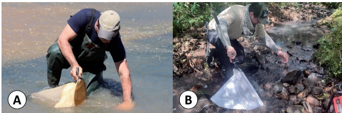
Figure 3 – Collection methods used in this study: A) surber type collector; and B) hand nets, applied manually. Source: Primary.
